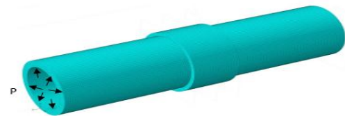
Figure 4 : Pipeline repaired under 100 MPa pressure load
